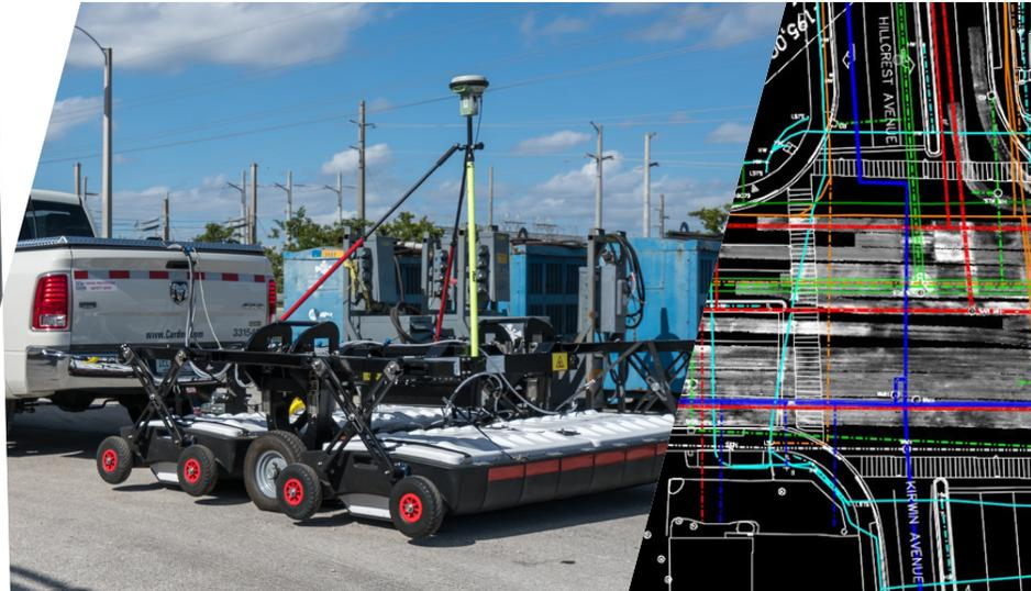
Understanding the locations of all utilities, both above ground and subsurface, is essential in managing utility risks. Using state of the art Multi-Channel Ground-Penetrating Radar (MCGPR) technology, our team can identify potential conflicts and help reduce risks.
