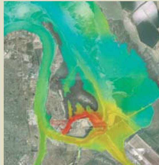
▲ Advanced modelling techniques can predict changes in water temperature as seen in Adelaide's Port River
