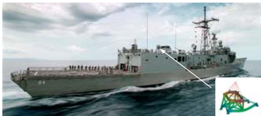
◀ FFG Class Frigate with deformed shape of radome support structure under transverse shock insert.
